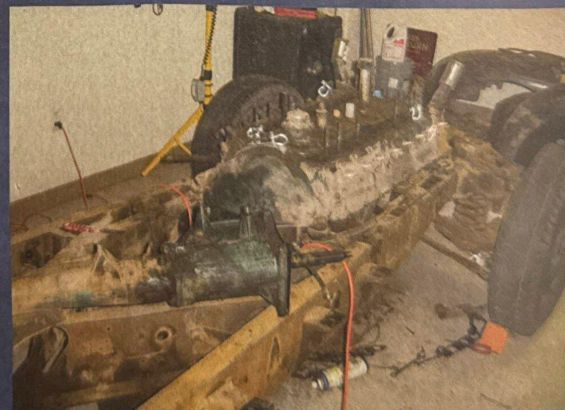
Afterwards, the chassis was rolled into Ken's garage, where he could begin its total disassembly. Here, the three-speed manual transmission has just been separated from the V-16 engine.
