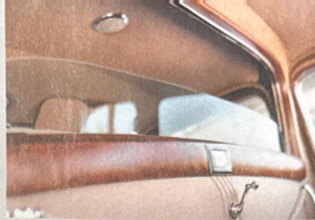
Separating the driver from passengers is a single-pane roll-up window that provided superior conversation privacy.
