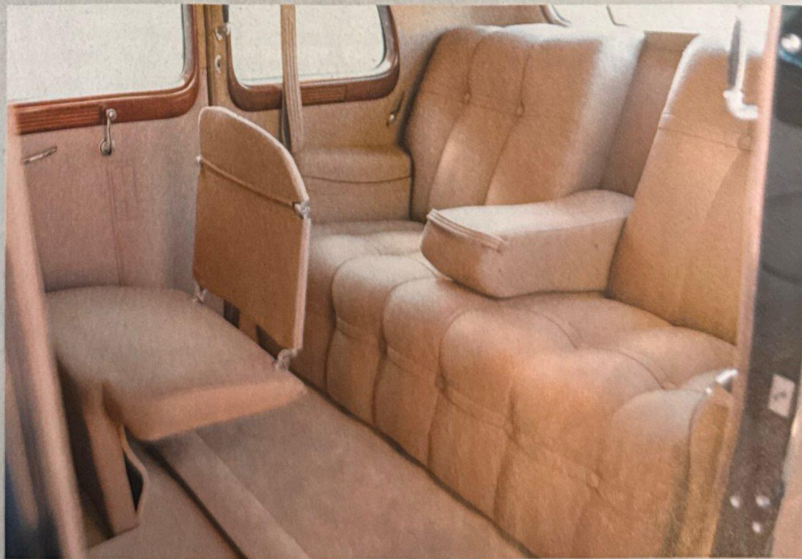
Cadillac's V-16 Imperial Sedan is listed as a seven-passenger vehicle, made possible through the provision of two collapsible jump seats, which themselves are finished as elegantly as the rest of the rear passenger compartment.
