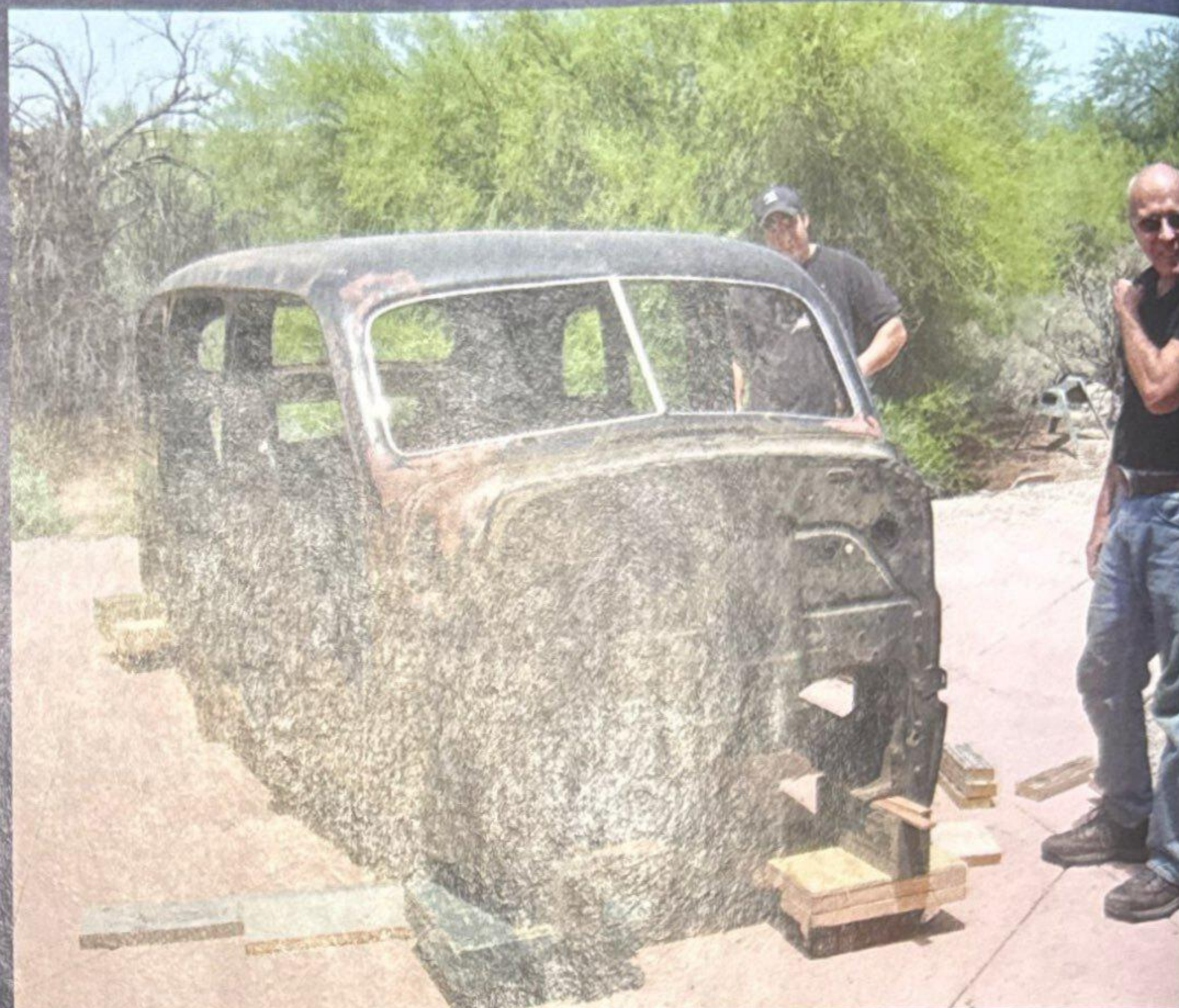
With the help of friends and fellow Classic Car Club of America members, Ken was able to separate the Cadillac's body from the chassis.
