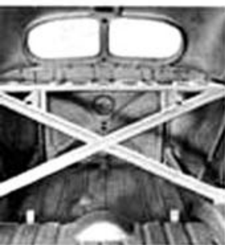
STEEL BRACING . . . A rigid "X" bracing is used across the back of the rear seat of all sedan models increase body rigidity.
