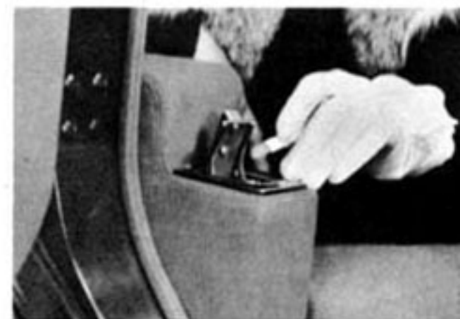
Ash receivers are located in each of the rear seat arm rests in addition to the one located in the center of the instrument panel.
