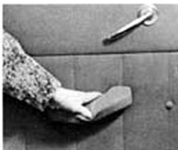
FLEXIBLE ARM RESTS . . . all hard reinforcing material has been removed from front door arm seats . . . door controls are formed so that the possibility of getting one's coat sleeve caught has been practically eliminated.
