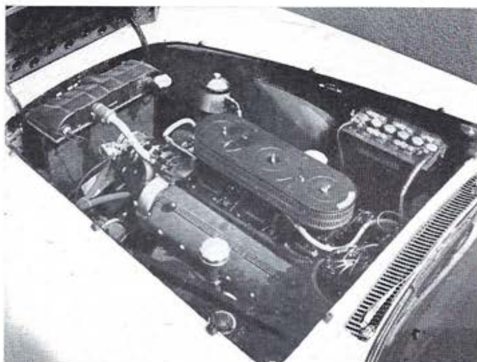
The power behind the throne; a 2953-cc V-12 sohc engine.
