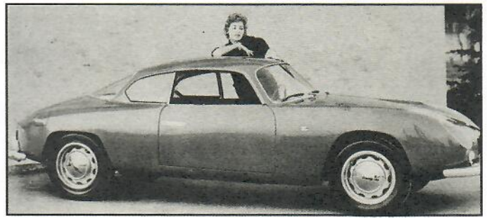
The GTE (early). One of Zagato's prettiest designs, at 40 inches high it's 8 inches lower than the Appia Sedan. Note the covered headlights and flush-mounted door handle.
