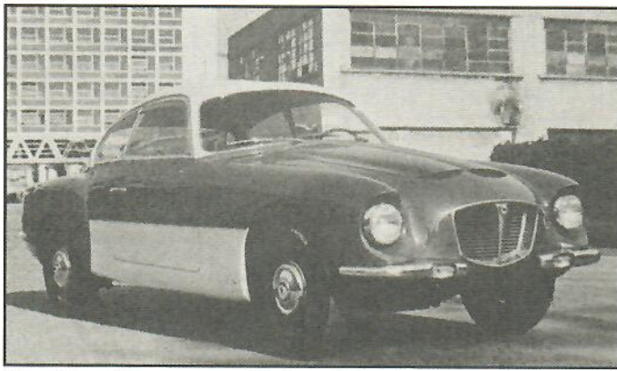
The "Camel" prototype. Distinguishing features include the two-tone color scheme, the traditional Lancia shield-shaped grille, and the split bumpers with recessed turn signals.
