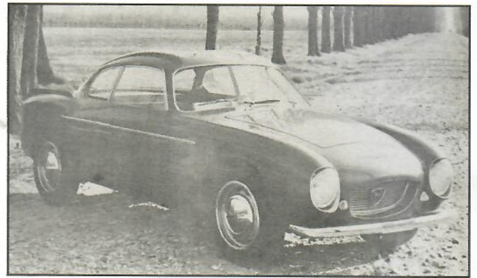
The GTZ. Note the "double bubble" roof, the covered headlights, the fins on the rear fenders, and the body side molding.
