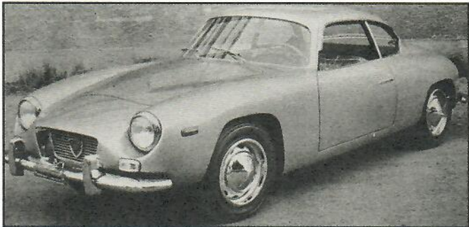
The GTE (late). The headlights have been moved slightly forward and are no longer covered.
